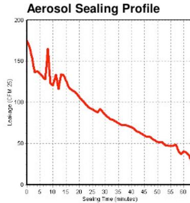
**Your Heating and Cooling Capacity Improvement for Duct Sealing is 20% based upon measured leakage reduction and original register flow**
